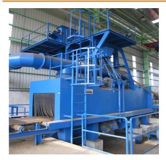
**SPEEDO AUTOBLAST Q1010** is the most appropriate surface treatment equipment for blasting raw steel profile & pipe external surface available in the surface preparation industry.
