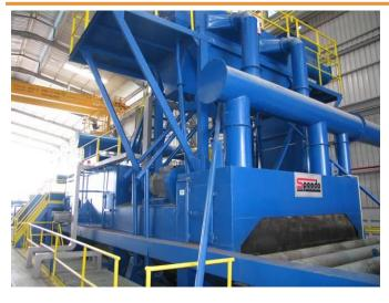
SPEEDO AUTOBLAST Q6930 is the most appropriate surface treatment equipment for blasting raw steel plate external surface available in the surface preparation industry.
